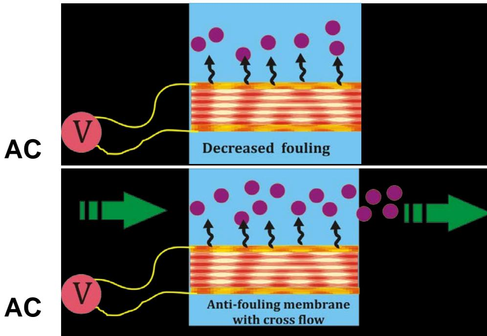
Electrically energised membranes would experience less fouling and have higher fluxes than passive membranes. This is illustrated in the figure below, where the flux through a piezo-electric membrane is plotted with and without application of the AC signal.
